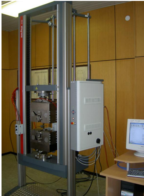
Figure 7. Computerized materials testing machine Zwick/Roel Z/100 Z 100
